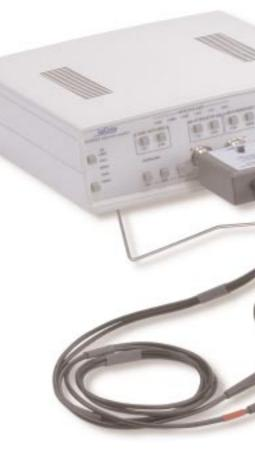
The AP015 current probe measures the current flowing through a conductor. The probe is based on a combination of Hall effect and transformer technology that allows measurements to be made on DC, AC, and impulse currents. Its rugged design uses a split-core transformer that allows the probe head to be clamped around a conductor that remains in circuit.
